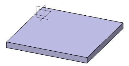
Using the Point icon, create a point at 1.75, 1.75, 0.25. This will be used to locate the sketch origin of the cutout. This will allow you to have this point as an input when the power copy is instantiated.
