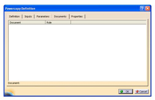
**Select the** *Properties* **tab.** The window should appear similar to the one shown below. This window will allow you to choose an icon to represent the power copy as well as attach a preview via a screen shot.
