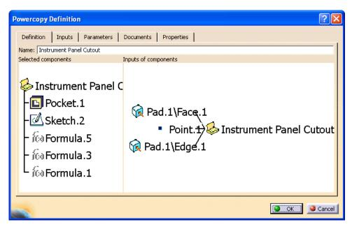
This window displays all of the inputs that were used to create the pocket. It is a good idea to give the inputs proper labels so that another user will have an idea of what they are defining upon instantiation.
