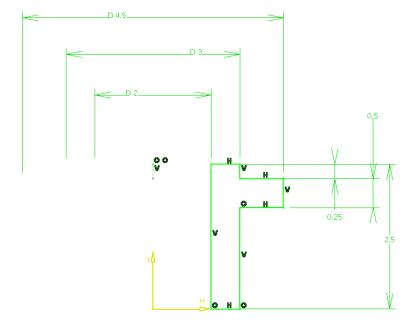
**Press the third mouse button while on the 2 inch diameter constraint and select** *Offset.17 object* **and select** *Edit Formula*. The *Formula Editor* appears. Notice that the parameter is really a radius and not a diameter even though it shows as a diameter in the graphical area.
