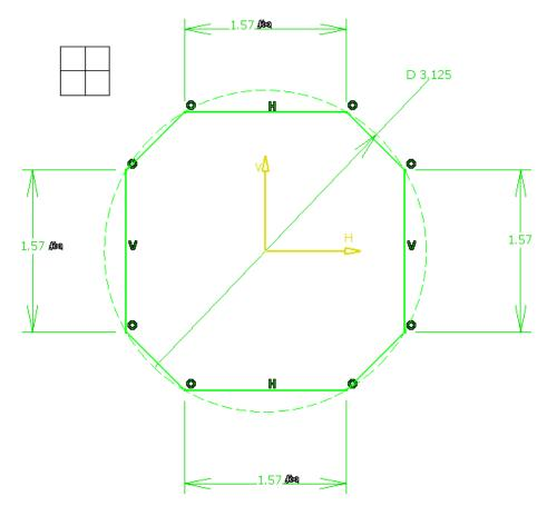
Exit the sketch and create a pocket, using *Up to last*. It should appear as shown below.
