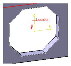
Select the *Parameters* button again and change the *SIDE\_LENGTH* to be 1.75 and select *Close* and then select *Preview* again. The cutout changes shape according to the specified parameters.
