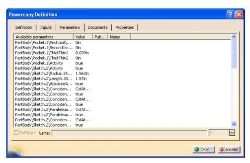
**Double select on the** *Radius* **parameter with a** *Value* **of 1.563in.** This parameter is for the radius of the circle used to constrain the sketch of the pocket. By double selecting on the parameter, you are activating it so it will be available for use when you instantiate the power copy later on. You can change the name of the published parameter at the bottom of the window.
