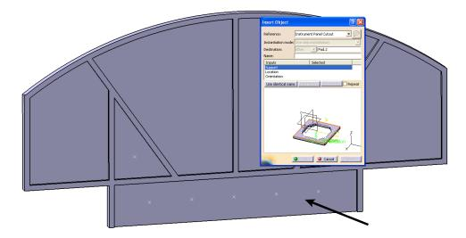
With *Location* selected, select the point on bottom left as shown below. It should automatically move to the *Orientation* input.
