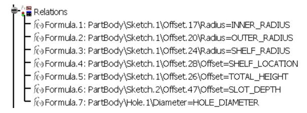
By setting the intrinsic parameters equal to the user defined parameters you can control the design by changing the user defined parameters.
