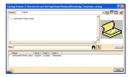
**Double select on the** *Instrument Panel Cutout* in the window. A *Warning* window appears. This lets you know that the formulas associated with the power copy will be inserted into your current document in a different location than the current location specified which is after *Pad.2*.
