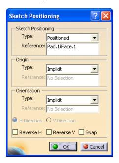
Under the *Origin* area, change the *Type* to *Projection point* and select the point that you just created. This locates the origin of the positioned sketch at the point.
