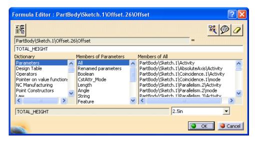
Notice at the bottom of the window is the driving parameter and its value appears. You can change the value at that location. Since this is a multiple value constraint you can choose a value from the list of available values.
