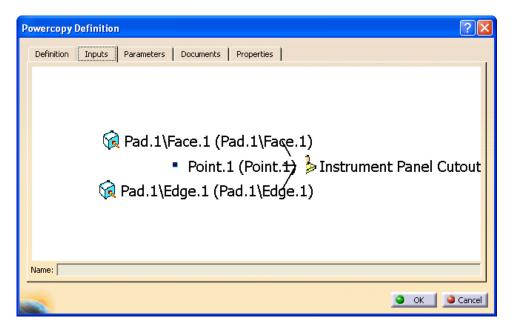
Select the first input in the window (This should be the face). You should notice this is the input specifying the sketch support for the pocket. It should highlight green in the display as shown below.
