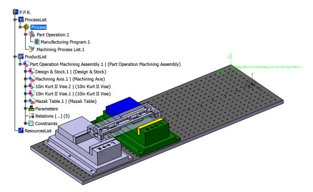
If you remember from the introduction, the prismatic machining workbench utilizes the PPR tree, the Process Product Resource tree. Refer back to the introduction for full details as to the PPR tree.
