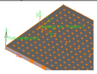
**Select** *OK* **to the machining axis window.** For now this will serve as the machining axis. Many times machine seeds will have an axis location defined that can serve as the machining axis.
