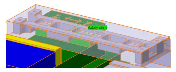
Granted, the top of the stock material is not a good location for the safety plane, however, the top of the stock material is the highest location on the assembly, therefore, it makes a good place to start from.
