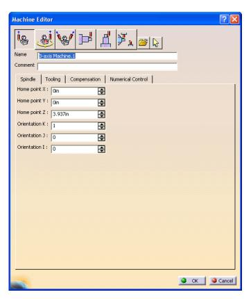
The first set of icons across the top allow you to define the specific type of machine you are going to be using.
