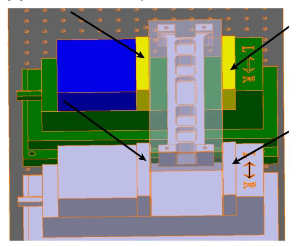
**Double select in the workspace when done.** You do not need to select on any part, just double select in space. You can define as many parts as fixture parts as you want. This will have four fixtures defined.
