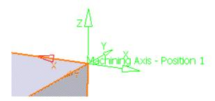
If you look very closely, you will notice faint red axis directions that indicate the new directions. Unfortunately, the green machining axis does not actually update until you complete the axis definition. You will find that many times you will need to complete the axis definition to insure the axis is correct. If it is not correct, then you will simply need to go back to the axis definition by selecting on the machining axis icon again.
