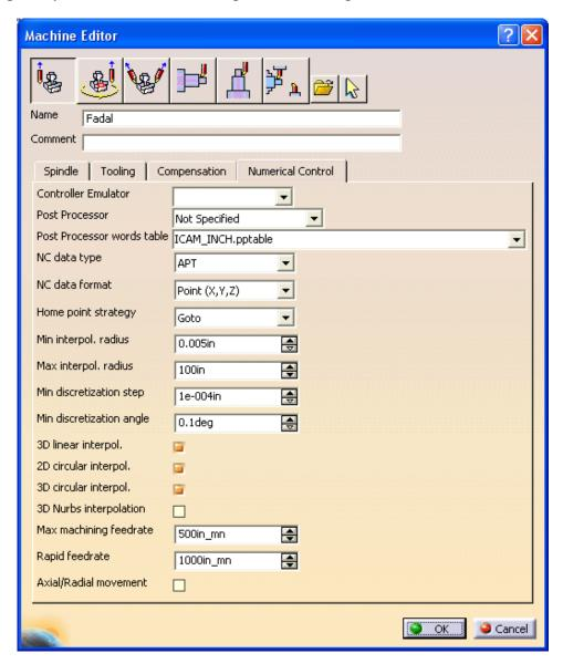
**Select** *OK* **when done.** This will have the machine set up.
