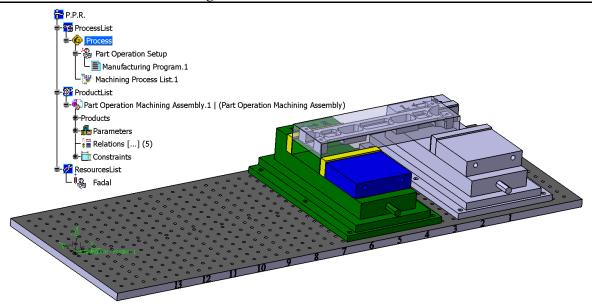
At this point, you are ready to begin defining machining operations to machine the part. Although this may seem like a long drawn out process, it is a mandatory sequence to go through each time you start a program. Failure to completely define the part operation will result in operations and macros having issues as you define them.
