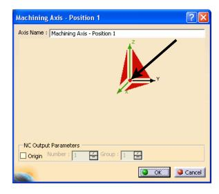
The center red dot will allow you to move the entire axis system from one location to another. The *Machining Axis System* window will disappear while CATIA waits for you to select a point or vertex to be the new center of the axis system.
