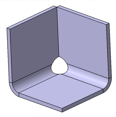
**Select the Fold/Unfold icon.** The part is unfolded.
