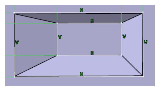
Notice the inner profile of the sketch matches up with the bottom edges of the stamp. This is because the inner profile of the sketch is acting as a punch for the stamp.
