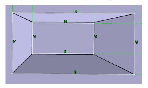
Notice the outer profile of the sketch matches up with the bottom outer edge of the stamp. This is because the outer profile of the sketch is acting as a die for the stamp.
