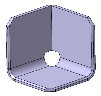
Notice the chamfer propagates around the tangent edges.
