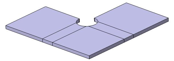
**Show** *Sketch.4* **from the specification tree.** You will replace the circular corner relief with a square profile corner relief using *Sketch.4*.
