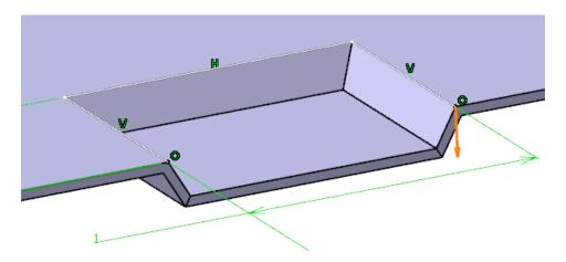
You should also notice that the upper edge of the stamp is located directly in line with the sketch profile. This is because the *Type* is set to Upward Sketch Profile by default.
