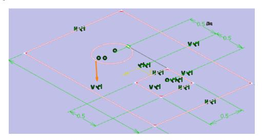
Set the Angle to be 80 and both Radius parameters to be 0.05.
