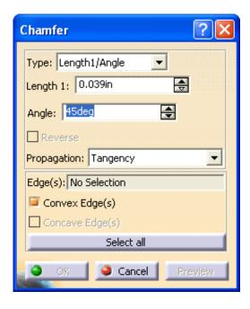
Specifies how the chamfer will be defined Type
