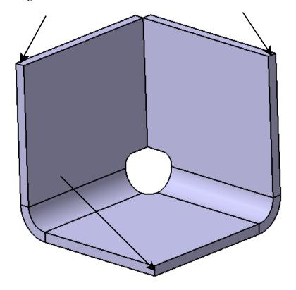
Set the Type to be Length 1/Angle and set Length 1 to be 0.25 and the Angle to be 45 and select OK. The chamfer is created.
