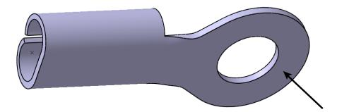
Select the centerline of the hole as the *Coincidence* placement constraint. Select *OK* when done. This will have the cavity connection point defined.
