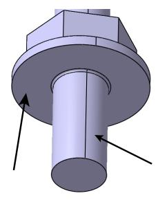
**Select** *OK* when done. This will define the necessary placement constraints for the stud mount. At this point, you are ready to start defining the other connection points.
