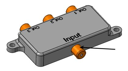
Select the front face of the connector as the *Contact* placement constraint. Again, this surface is shown.
