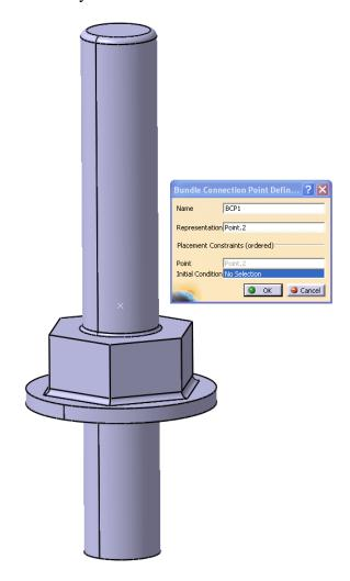
Notice that the representation and the point definition were defined just by creating the one point. When you select a point as the representation, the point placement constraint is automatically defined.
