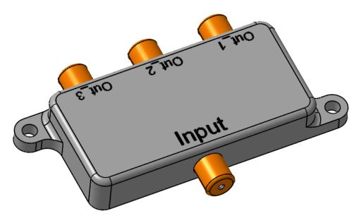
Using the Define Connector icon, define this part as a *Multi Insert Connector*. Change the *Part Number* to <u>Cable TV Splitter</u> and leave the *Number of Terminations* at zero and select *OK*. Even though you are going to end up defining eight terminations for this model (two per connector) you will be learning to define this after the fact for this connector.
