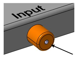
Select the centerline of the connector as the *Coincidence* placement constraint. This will have the connector connection point defined.
