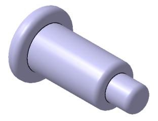
**Select the Define Filler Plug icon and select the filler plug.** This will display the *Filler Plug Definition* window. Just like a contact, only a part number change is available with the definition of a filler plug.
