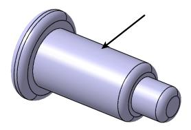
Select the ledge of the larger surface as the *Contact* placement constraint and the centerline of the filler plug as the *Coincidence* placement constraint. The contact placement constraint surface is shown below.
