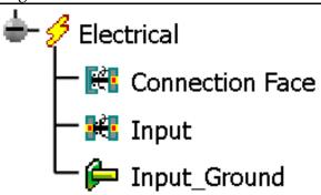
Using the Define Termination icon, define another termination for the tip. Set the *Id Number* to <u>Input Tip</u> and select the inner cylindrical surface as the *Representation*. This is shown below.
