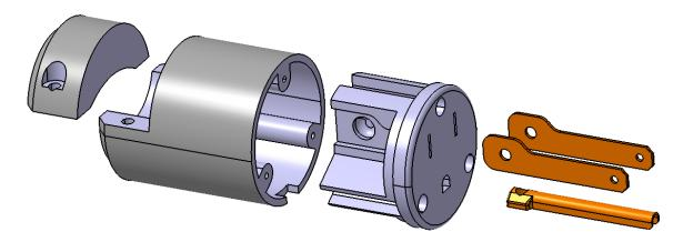
At this point, you would have a very high level of detail for both the digital design of the model and the electrical properties for this assembly. In this case, you would not only be able to define the contacts for the electrical part, but you would also be able to define the shells, back shells, supports, and all other components for the plug. Keep in mind, although this type of assembly does show and have the most detail, it also takes the longest to build.
