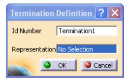
Look familiar? This is the same window that is displayed when you double select on a termination from the tree. If you remember, the *Id Number* simply defines the termination identifier and the *Representation* defines the geometry that will highlight when the terminal is selected.
