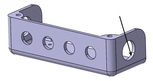
Create a point at the center of the hole as the *Point* placement constraint and select the planar face as the *Initial Condition* placement constraint. This will have the first bundle connection point defined for the external splice.
